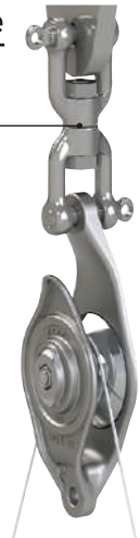
Improved strength through the integrated structure of the sheave shaft and main body. The edges of the sheave are designed to fit into the main body to prevent ropes from getting tangled.
