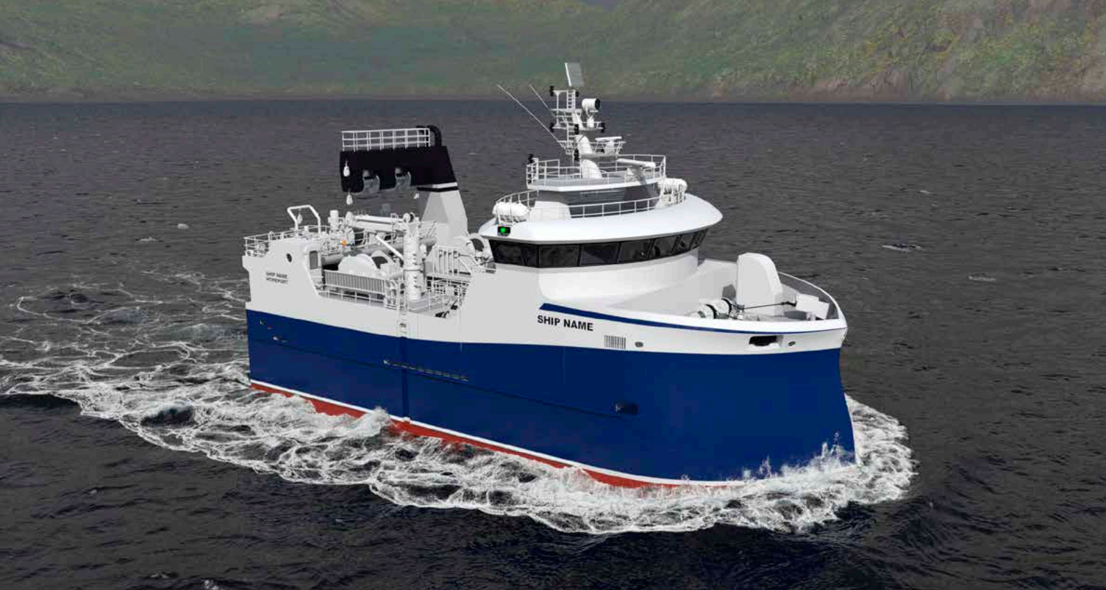
Nautic: 29m trawler outfitted with three trawl winches and is available in Methanol version and conventional diesel.
